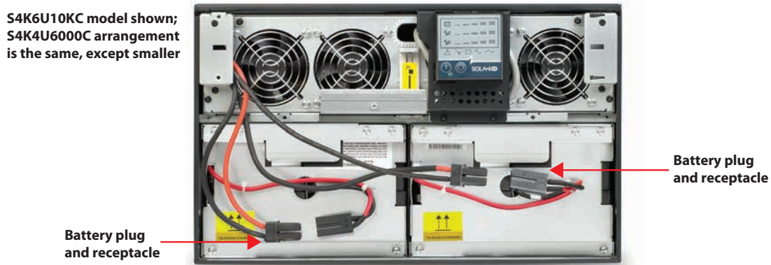
Figure 29: Disconnecting the battery plug and receptacle (front view)
